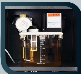
Lubricating Oil Pump
