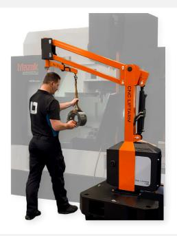
The CNC LiftArm is the perfect solution for the efficient loading and unloading of heavy workpieces in CNC- or other machines.
